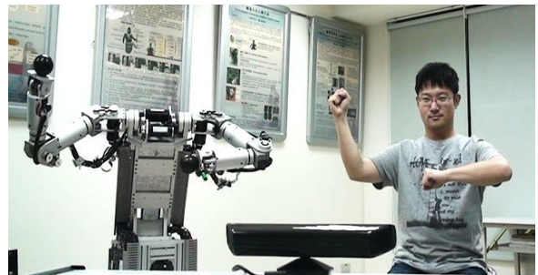
Fig. 1. The robot is controlled by human demonstration in real time using Kinect sensor.
